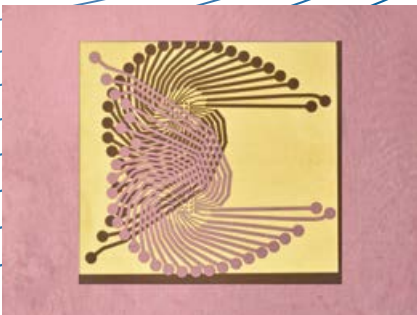
Removal of copper from double-sided PET film
