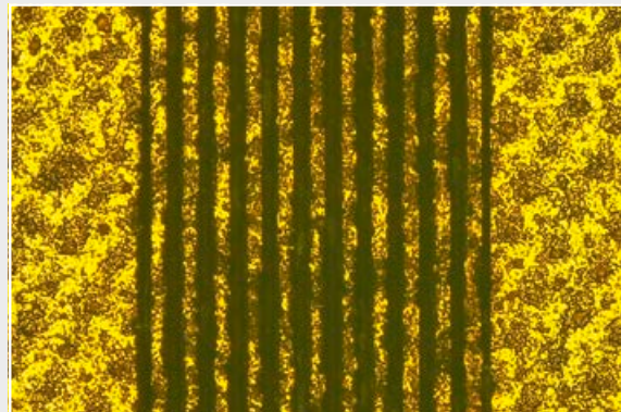
Structuring on \text{Al}_2\text{O}_3 with Cu/Au plating using the laser (50 \mu\text{m} traces/25 \mu\text{m} spaces)
